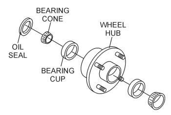
Figure 29. Wheel Hub and Bearings
